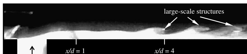
Fig. 5. Flow visualisation for Re_c = 13,000 (without grid turbulator).
